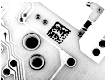
Figure 195. Data Matrix Code Directly Marked on PCB Surface by Using Laser Etching Technology
