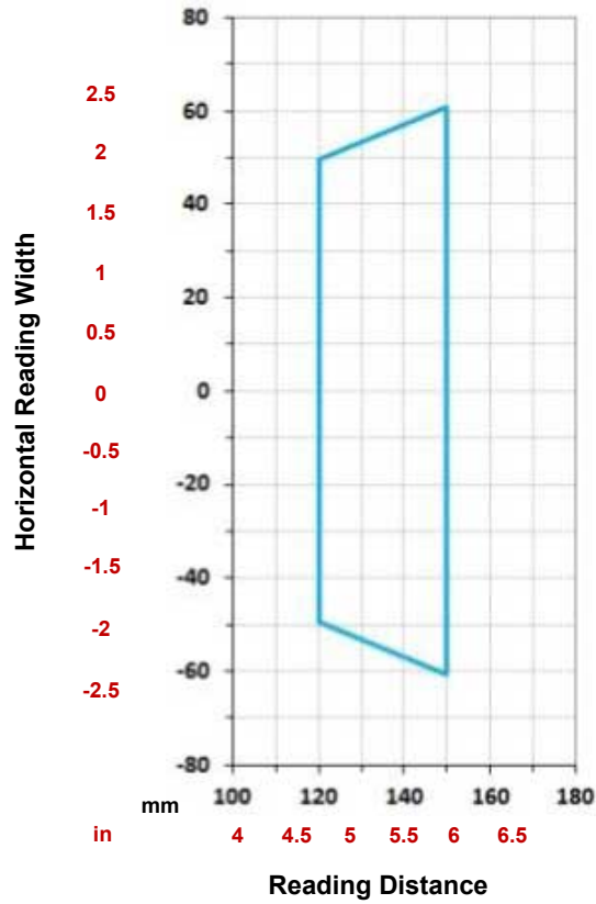
Figure 169. Data Matrix 0.19 mm (7.5 mils)
