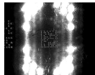
Figure 240. Multicolored DPM - Central Group: Incorrect Illumination
