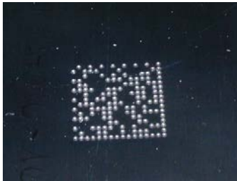
Figure 193. Directly Marked Dot Matrix Code Characterized by Outstanding Separation Distance between Adjacent Code Elements
