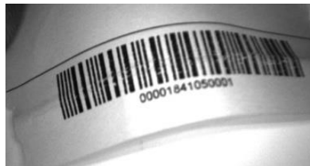
Figure 190. Barcode Printed on Curved Surface Readable by ABR in spite of Image Optical Distortion
