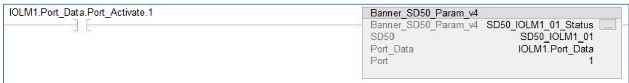
3. The final step is to place an examine on in front of the AOI. This is linked to the Port\_Activate for the port the device is plugged into. In this example that is IOLM1.Port\_Data.Port\_Activate.
