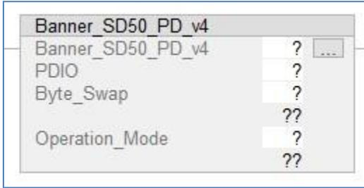
2. In the AOI, right-click on the question mark on the line labeled “Banner\_SD50\_PD\_v4”. Click New Tag. Name the new tag. This example uses the name “SD50\_IOLM1\_01\_PD\_Status”. The example naming convention accounts for this being an SD50 Pro device connected to IO-Link Master #1, port #1, in our program. More masters could be named IOLM2, IOLM3, and different sensors could be connected at other port numbers, etc.
