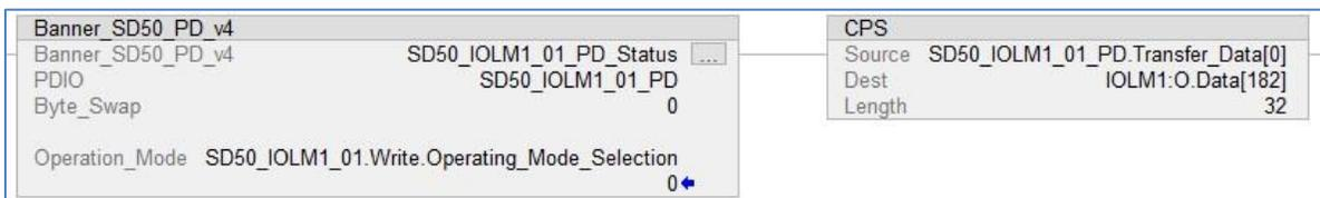
If a Banner IO-Link Master is being used, setup a Move block. Send a 1 to the Activate Outputs array value (see table for each port's value). As an example, if port 1 needs the process data outputs active then send a 1 to 181.
