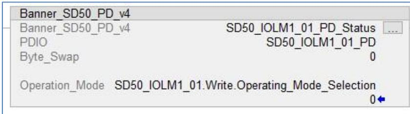
NOTE: if you type in the incorrect number (i.e. it does not match the device’s current configuration) you will get incorrectly displayed Process Data Out information.
