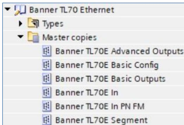
4. Create one Output (Required) Tag and 2 Input (Optional) Tags under PLC Tags. Link the Outputs tag with the Data Type "Banner TL70E Advanced Outputs". Link the inputs as shown in the image.
