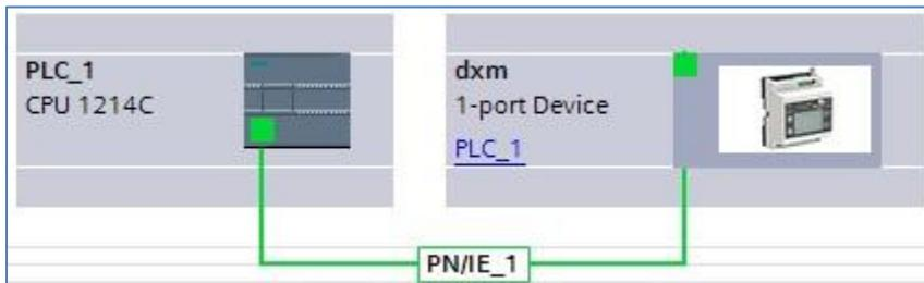
3. Go to Device View. Configure Slot 7 with 256 bytes integer output. The connection should look something like the below image. The Output addresses shown will be used for this example. This is the only link that is needed to control the TL70 Ethernet light.
