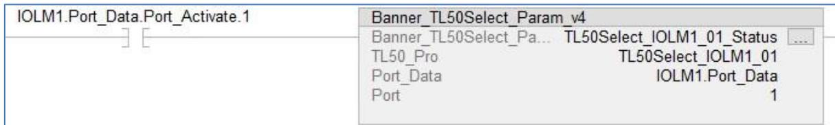
3. Finally add an Examine ON to the beginning of the line that the Parameter AOI is on. Tie this to the IO-Link Master AOI’s “Port Activate” bit corresponding to the port number to which the TL50Pro Select is connected. In this example, the TL50 Pro Select is on Port 1 of the IO-Link Master named IOLM2, so the bit “IOLM1.Port\_Data.Port\_Activate.1” is used.
