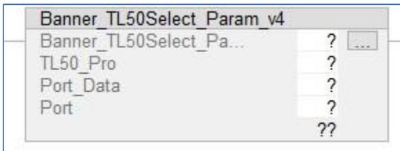
2. In the AOI, right-click on the question mark on the line labeled “Banner\_TL50Select\_Param\_v4”. Click New Tag. In this example, we’ll use the name “TL50Select\_IOLM1\_01\_Status”. The example naming convention accounts for this being a TL50 Pro Select device connected to IO-Link Master #1, port #1, in our program. More masters could be named IOLM2, IOLM3, and different sensors could be connected at other port numbers, etc.
