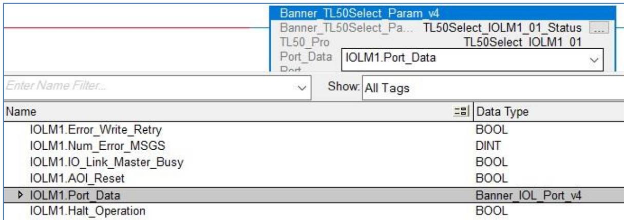
2. For the last line of the TL50 Pro Select AOI, “Port\_Number”, type in a number equal to the IO-Link Master port number to which the TL50 is connected. In this example, the device is on port 4.
