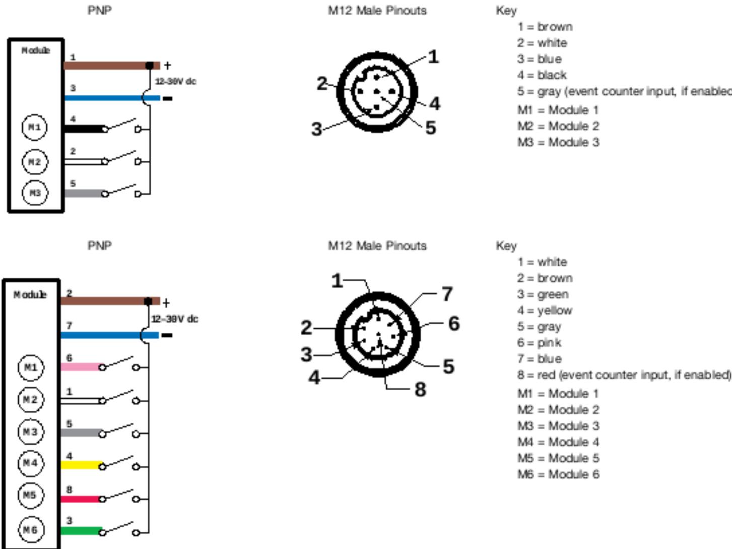
Input wires M1 through M6 can be used to either control the light segments or can be configured as external PNP Inputs. Refer to [Set the Radio Module DIP Switches](#) on page 3 for configuration instructions.
