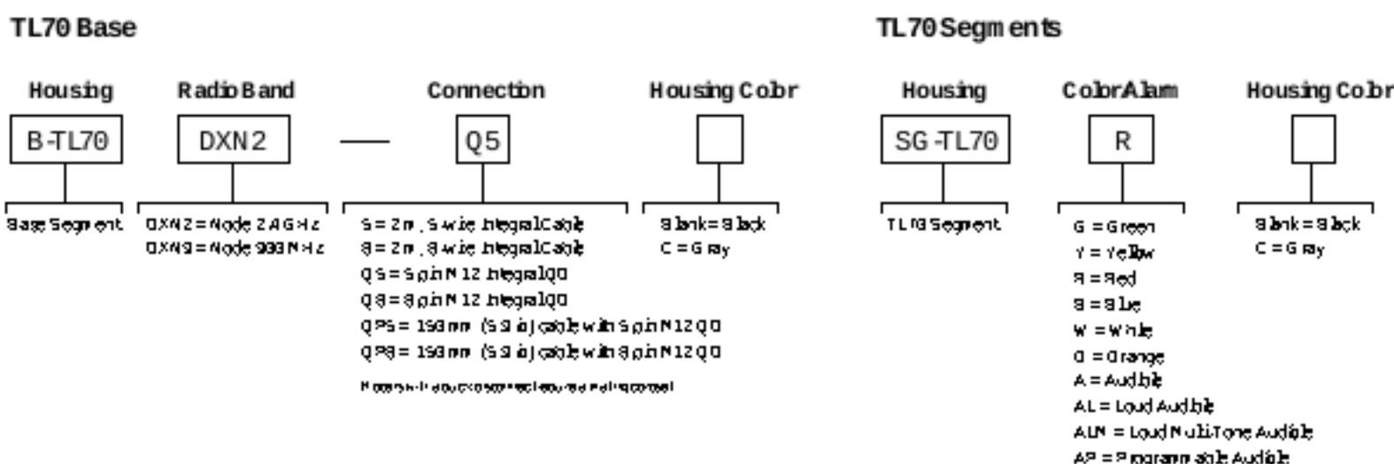
Select the 5-pin base for tower light configurations of up to three modules. Select the 8-pin base for tower light configurations of up to six modules.
