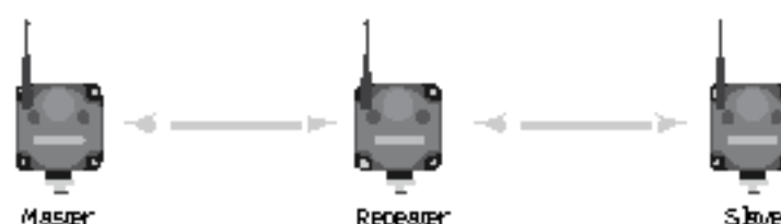
Figure 3. Point to point network with repeater
