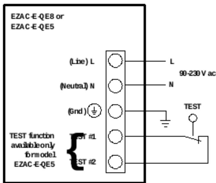
Figure 13. Wiring—model EZAC-E-QE8-QS3 (3-pin Mini-style QD)
