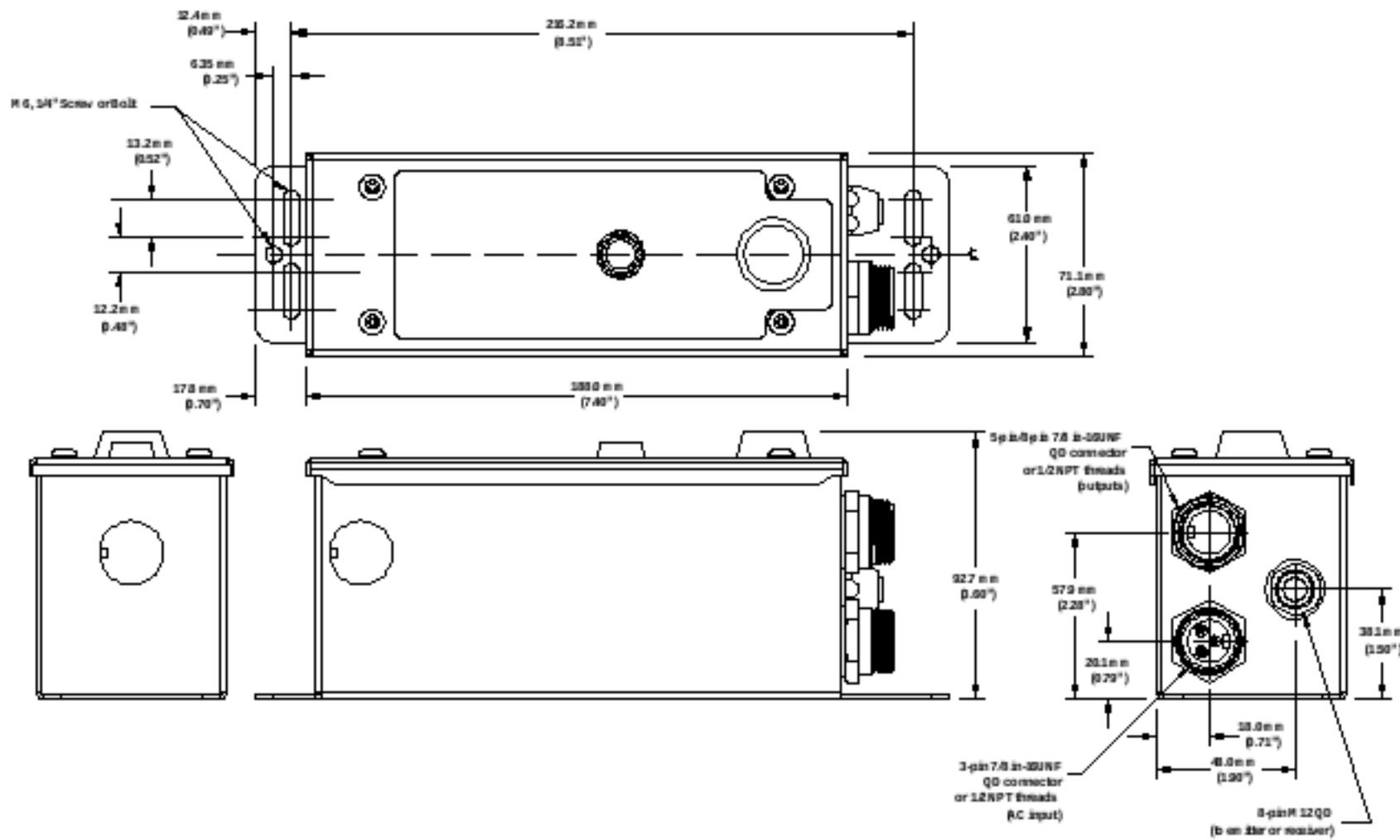
Figure 17. Model EZAC-E.. EZ-SCREEN AC Interface Box
