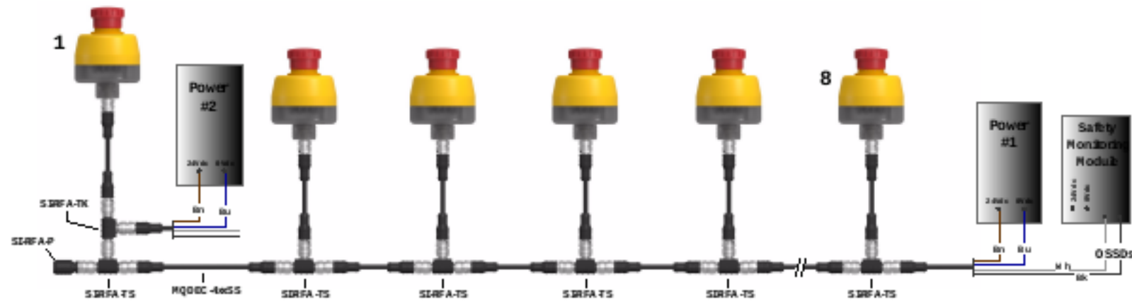
Figure 10. Option 2: Replace the terminator with a power supply. The O5SD1 and O5SD2 wires at power supply #2 must be connected to +24 V DC. If available set the power supplies for parallel output.
