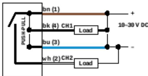
Figure 2. Channel 1 = IO-Link, Channel 2 = PNP Remote Input
