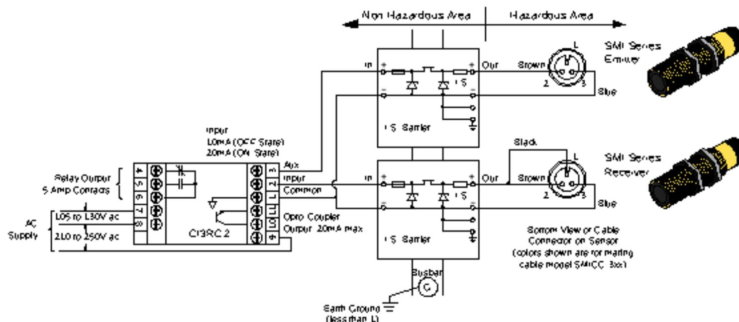
Figure 4. Hookup Using One Dual-Channel Barrier
