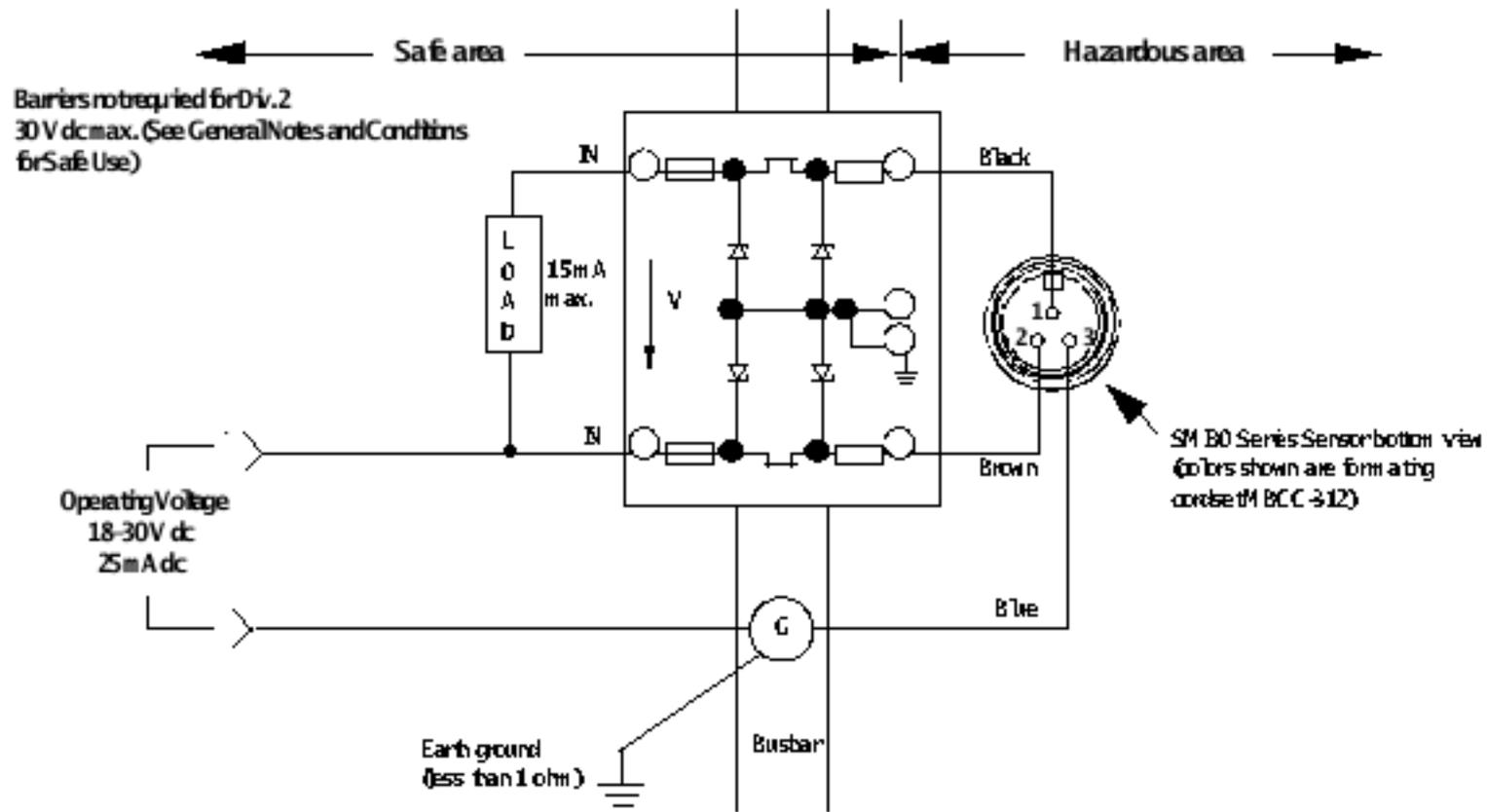
Note: Emitters have no output connection (no connection to black wire)
