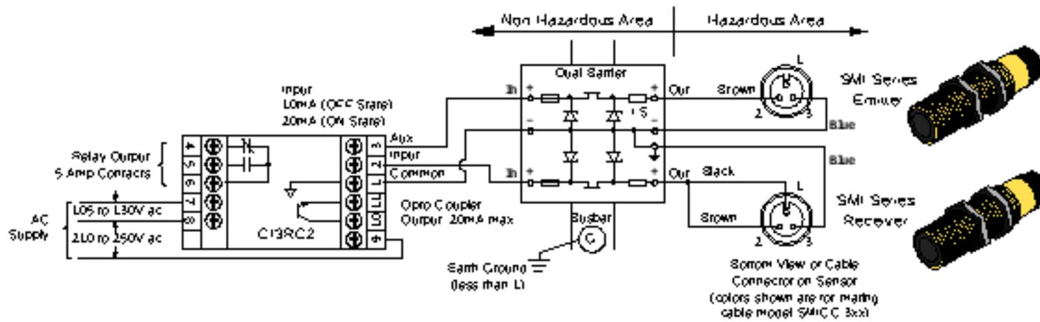
Both sensors of the opposed mode pair are wired to model CI3RC2 using the two-wire hookup, which requires the use of two single channel or one dual channel intrinsic safety barrier(s). In this mode, the SMI30 receiver sinks less than or equal to 10 milliamps in the "OFF" state and greater than or equal to 20 milliamps in the "ON" state. The CI3RC2 senses this current change and switches internal relays that are easily wired to most loads and/or additional control circuitry.
