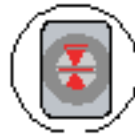
Figure 7. Tension Indicator Window: proper tension shown
