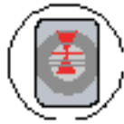
Figure 6. Tension Indicator Window: too little tension shown
