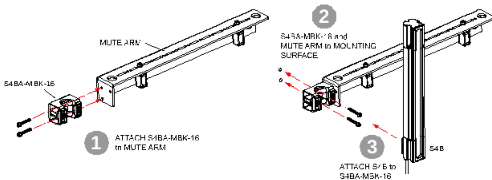
3. Attach the mute arm to the side of the bracket with the user-supplied M4 hardware.
