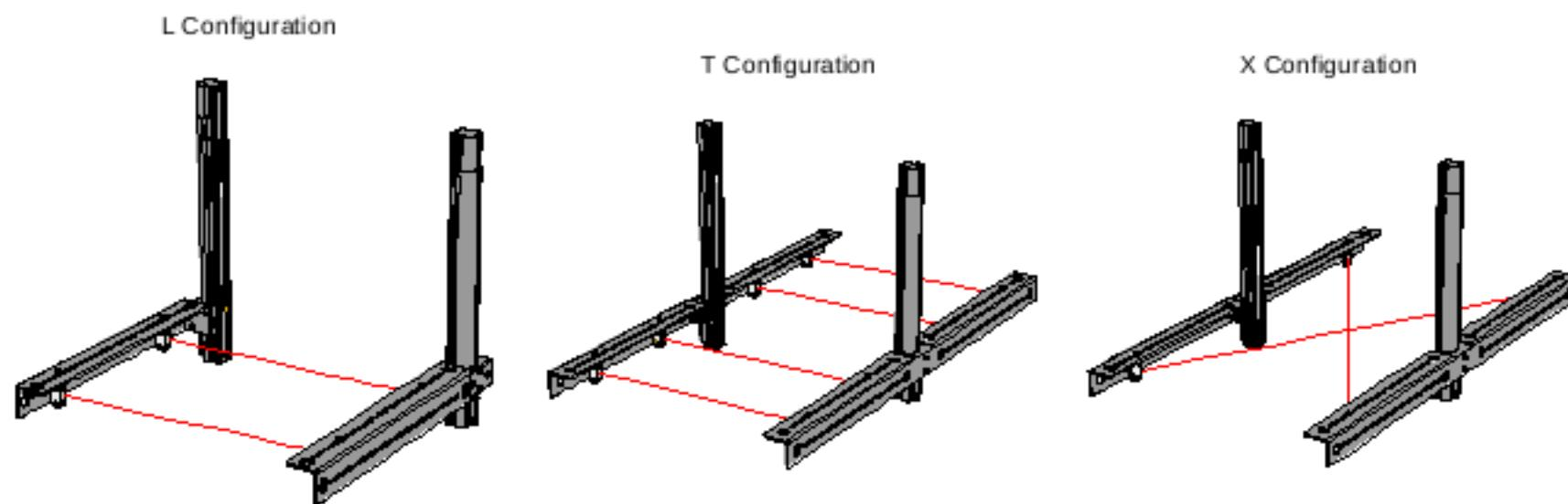
The S4B Mute Arm Sensor Kit can be directly mounted to a flat surface. The kit can also be mounted to the S4B Safety Light Curtain system's mounting brackets, S4BA-MBK-16 (or for the T and X system, directly to a stand). Connect the included Q20-2 sensors and the light curtains to the muting device. The use of an appropriate molded junction block, such as R95-6M125-M128-S4BM, can simplify wiring.
