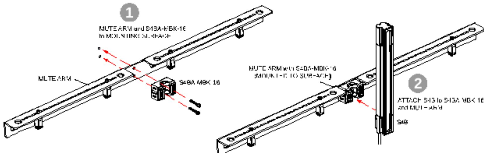
3. Mount the S4BA-MBK-16 bracket and the mute arm bracket by placing the S4BA-MBK-16 on the mute arm bracket and attaching it to the mounting surface.
