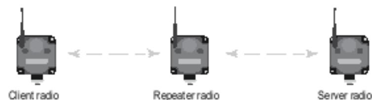
Point to point network with repeater for cable replacement applications
