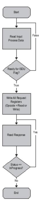
The request is dispatched to the connected device after the request is written. For a read operation, at the end of the sequence, the response data contains the data returned from the device.
