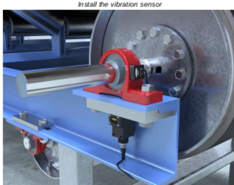
Magnets are slightly less effective but provide more flexibility for future adjustments and faster installation. Magnet mounts are susceptible to accidental rotation or change in the sensor location if an outside force bumps or moves the sensor. This can lead to a change in the sensor information that differs from the time-trended data from the previous location.
