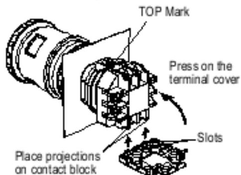
3. Press the SSA-EB1-TC terminal cover toward the contact block.
