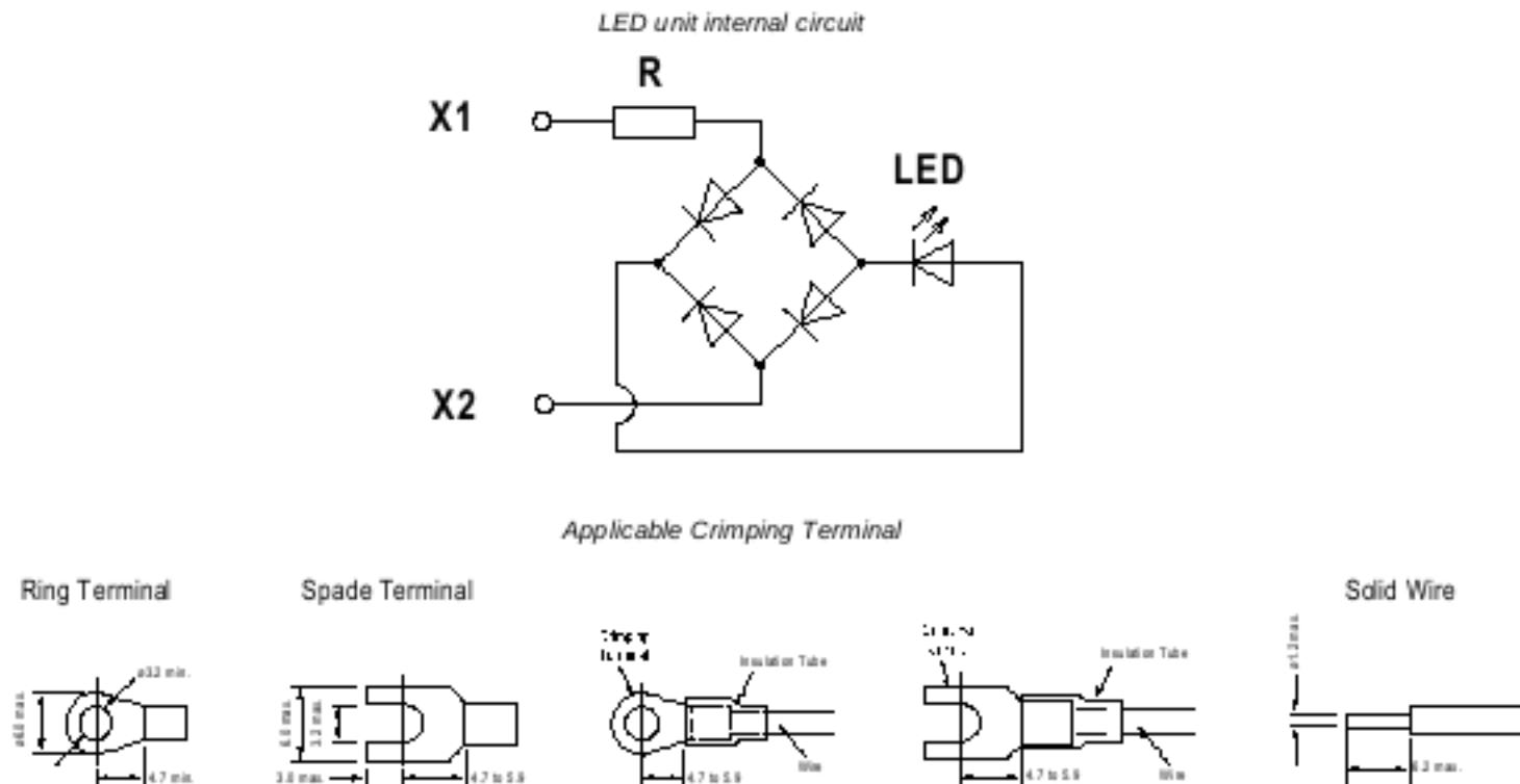
Banner recommends the use of crimp terminals with stranded wire or solid core wire to prevent short circuits between terminals. Ensure that the insulation tube is installed on crimp terminals.
