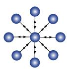
Pros—The gateway maintains a communications connection with each node on a separate communications path; if communication between one node and the gateway fails, the rest of the network is unaffected; and chattering nodes are removed from the network.
