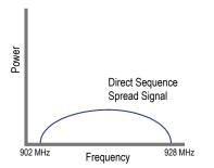
The DSSS encoder spreads the data across a broad range of frequencies using a mathematical key. The receiver uses the same key to decode the data. Although narrowband and DSSS transmissions use the same total power to send data, DSSS uses a lower power density (power/frequency), making it harder to detect. DSSS also sends redundant copies of the encoded data to ensure reception.
