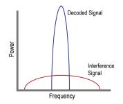
The DSSS signal uses a much lower power density than narrowband inference.
