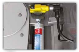
The QS18U ultrasonic sensor can work adjacent to the FI22 sensor. Thanks to its retrosonic set-up (which uses the background as a reflector) it can reliably detect the tube irrespective if this is opaque, transparent, glossy or coloured.
