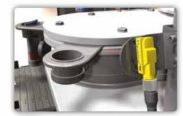
The QS18FF sensor is a background suppression sensor with fixed range and can be used ideally to check if a tube has been ejected at the end of the sealing process thus eliminating the need for a reflector.
