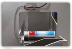
The FI22 fiber optic sensor is IP67 and can be mounted adjecent to the application without additional protection. It checks the orientation of the empty tube by detecting the presence/ absence of the cap.
