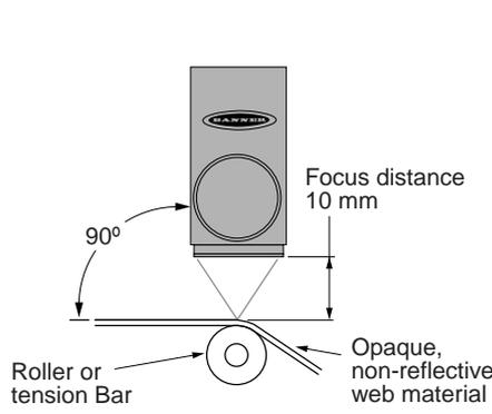
Fig. 1 Mounting for sensing opaque non-reflective materials
