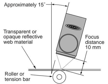
Fig. 2 Mounting for sensing opaque reflective and transparent materials
