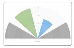
The 120 deg x 40 deg field of view is highly configurable and enables precision positioning and control
