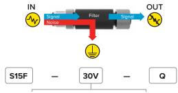
**30V** = 30 V DC voltage suppressor **H-500** = Hi-impedance filter 500 mA max
