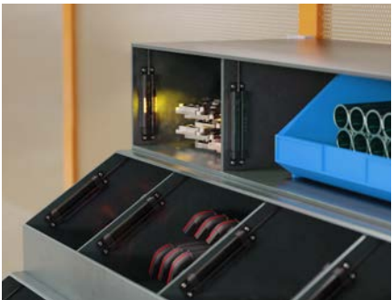
PVS sensors create a 2D detection field that can detect when someone reaches inside a bin to pick a part.
