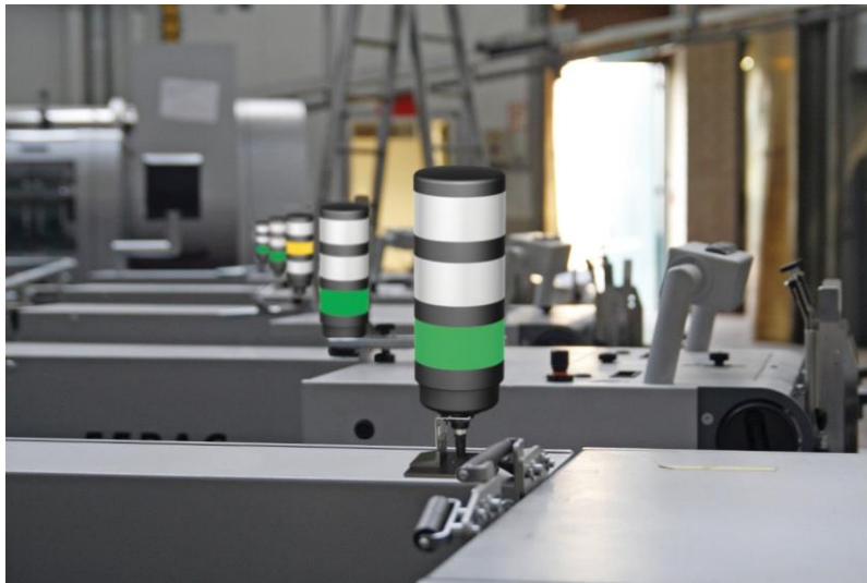
IO-Link reduces wiring for easy setup of devices, such as tower lights
