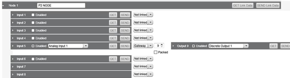
5. Click SEND Link Data on the Node 1 line to send the I/O linking information back to the devices.
