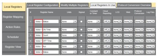
To display the motor status, count, or timer on the website, change the **Cloud Permissions** drop-down list to **Read** for each motors' information piece (status, Timer, count, etc.).
