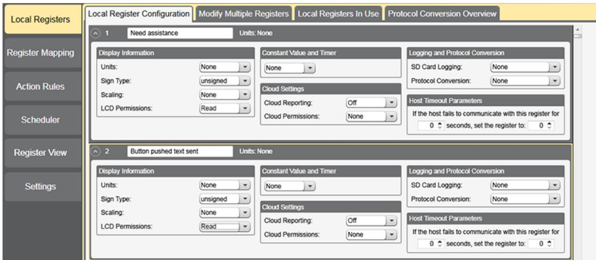
1. Launch the DXM Configuration Tool software and select the Local Registers screen.
