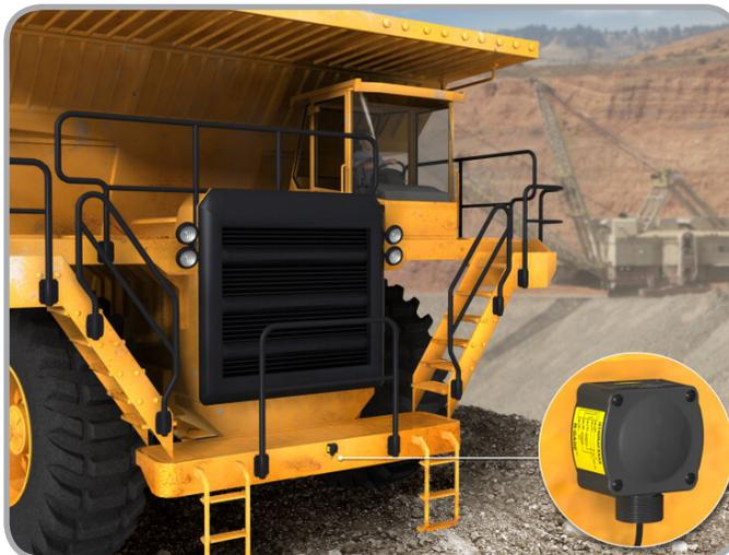
R-GAGE™ adjustable field radar sensors deployed on the front and back of dump trucks used at a surface mining site are an integral component in the vehicle's collision avoidance system
