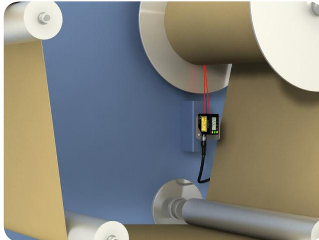
An L-GAGE<sup>®</sup> LE550 laser gauging sensor provides continuous roll diameter measurement for paper table coverings in a broad pallet of colors and regulates unwind speed
