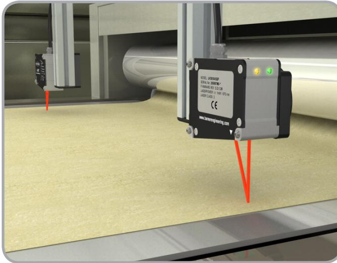
L-GAGE<sup>®</sup> LH Series Laser Sensors deployed on the sprout line measure dough height prior to baking
