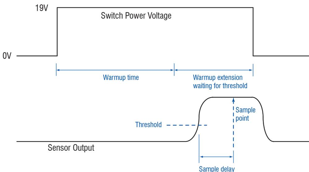
The switch power output is activated for the time defined by the warm-up time parameter. The device looks at the input to see if it is above the threshold setting.
