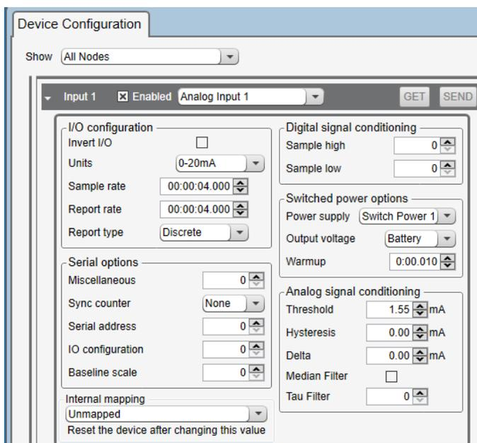
8. Click the arrow to the left of Node 1 to expand Node 1's parameters. Input 1 should be enabled, set to Analog Input 1. Verify the units are set to 0-20 mA.
