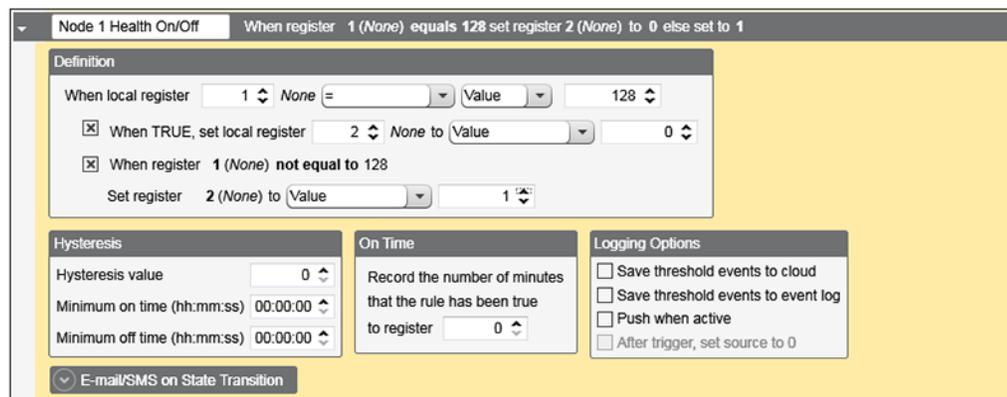
This threshold rule sets local register 2 to 0 when Node 1 is in the network and sets local register 2 to 1 when Node 1 has dropped out of the network. Use local register 2 to turn on an LED when the Node has lost its radio link with its master radio.
