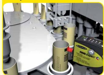
**Objective:** To detect registration marks on tubes for correct positioning before filling.
