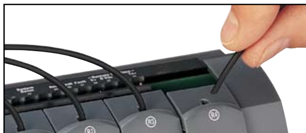
Figure 3-2. Installing the prepared fiber ends into the controller
