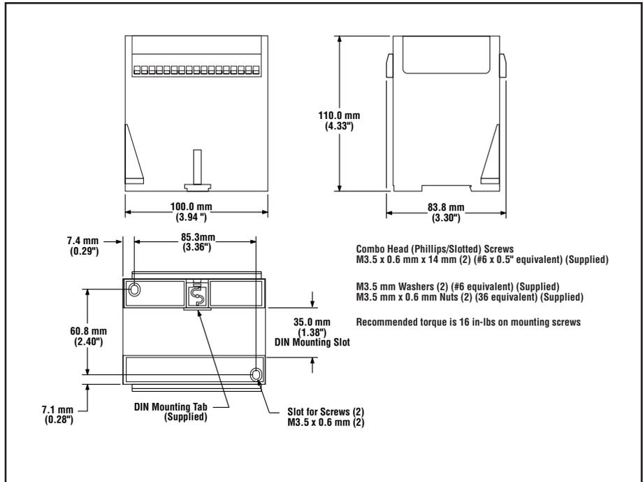
Figure 17. Control Module Dimensions and Mounting Hole Locations.
