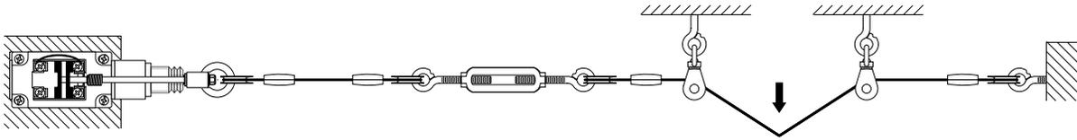
Figure 3. Rope Break or Slack: Contact 13-14 Opens
