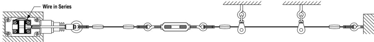
Figure 2. Rope Pulled: Contact 25-26 Opens
