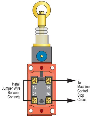
**Access to the Wiring Chamber.** The wiring chamber is accessed via a cover plate (remove two screws). A conduit adapter is supplied to convert the 20 millimeter threaded entrance to 1/2" NPT. An accessory cable gland which fits the M20 thread is also available.
