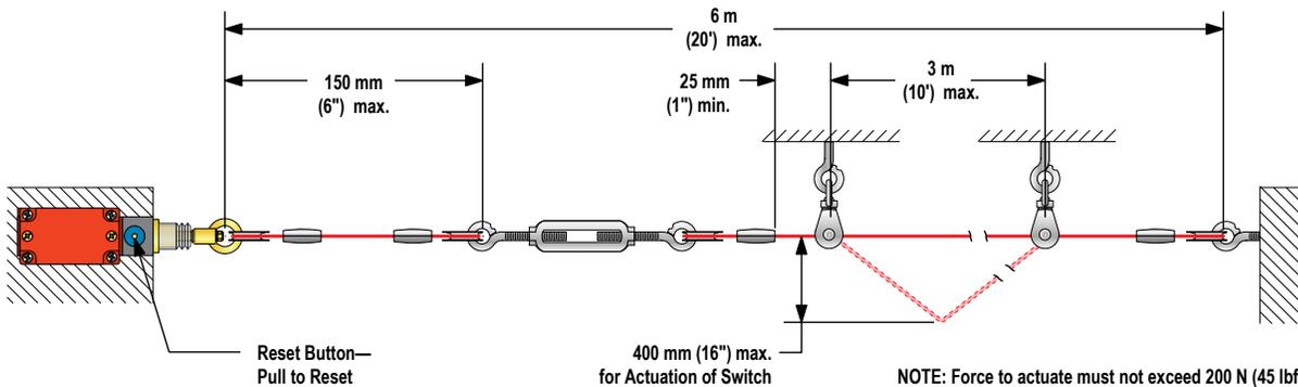
All hardware is supplied by the user. The switch mounting holes are on a standard limit switch mounting pattern of 30 x 60 millimeters, and accept M5 (#10) hardware. Wire rope and associated hardware may be ordered separately; see [Accessories](#) on page 6.
