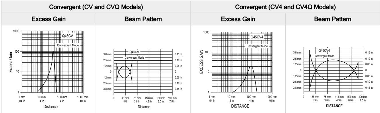
Glass fiber optic diffuse mode performance curves are based on a 90% reflectance white test card.
