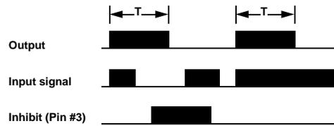
A ONE-SHOT output is a pulse of adjustable "hold" duration. With the module programmed for LIGHT operate, the pulse occurs when the input signal changes from dark to light. In DARK operate, the pulse occurs with a light-to-dark transition. Grounding pin #3 prevents the one-shot from triggering, but does not affect a pulse already underway.
