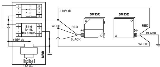
The SM53E/SM53R sensor pair has an analog output which serves as the input to a B4-6 ac-coupled amplifier. Note that the white wires from both emitter and receiver tie together at the amplifier input. This connects together the AGC circuit which regulates the emitter output for constant received light signal strength. The model MRB chassis (shown) operates from 120V ac and provides +15V dc to the sensors and amplifier module.
