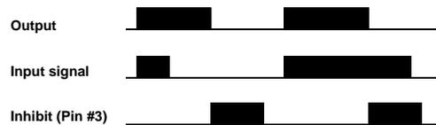
An AC LATCH is a combination of a ONE-SHOT and a LATCH. A light-to-dark or dark-to-light transition (depending upon the the LIGHT-DARK operate switch position) will latch the output "on". Grounding pin #3 will reset the latch.
