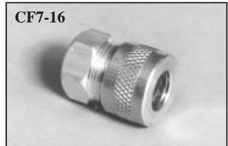
Aluminum compression fitting for the cable entrance at the rear of the 512 Series sensors. May be used with either plastic or flexible steel conduit (PVC-6 or AC-6).
