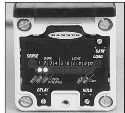
DARK condition example: D.A.T.A. system LEDs #1 and #2 lit.
