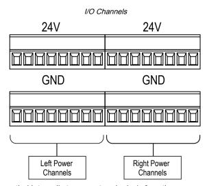
The left and right power channels are tied internally to screw terminals 1–3 on the power supply screw terminals.
