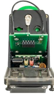
1. Loosen the clamp plate with a small Phillips screwdriver and lift the cover.
