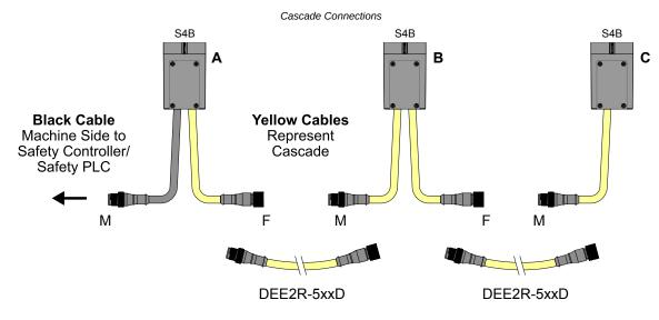
RD (removeable disconnect) cordsets A are either DES4-M51-F51-D (5-pin machine cable) or DES4-M81-F51-D (8-pin machine cable), depending on the kit ordered. Install these on the host emitter and receiver of the cascade system.
