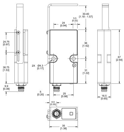
The EG24 can be ordered without the retroreflective arm or the arm can be removed for mounting flexibility. In either case, the provided retroreflective tape must be used and must be mounted 30 mm to 40 mm away from the lens to ensure optimal performance. If a replacement reflector is needed, contact Banner Engineering.
