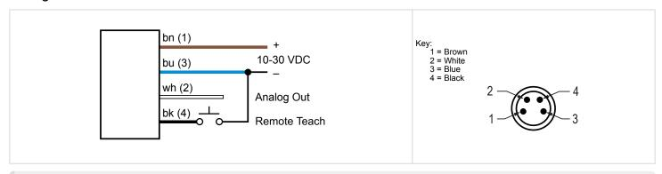
NOTE: For model EG24-ILVA-Q7B, the analog output is on the black wire (pin 4) and the remote teach is on the white wire (pin 2)
