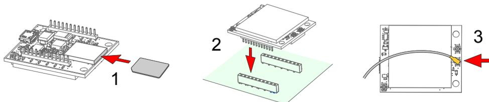
1. SIM cards come in a credit card sized carrier. Carefully snap it out of the carrier.
