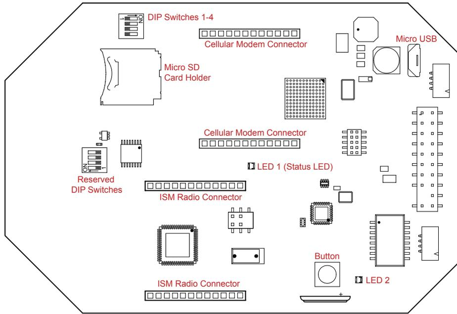
DXM Controller base board, cellular modem board, and ISM radio board
