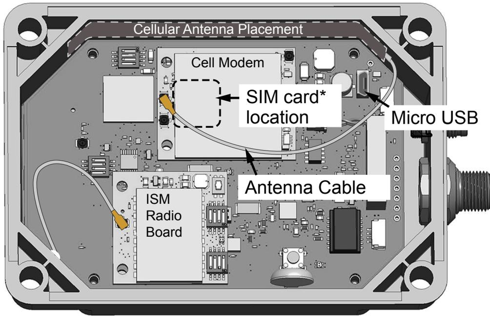
\*SIM card is located on the underside of installed modem
