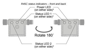
\* Indicator LEDs are visible through translucent housing
