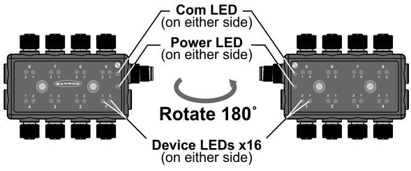
LED 1 = Discrete 1 In/Out LED 2 = Discrete 2 In/Out
