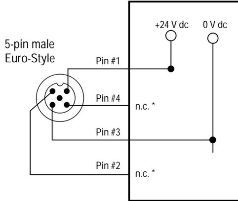
\* All pins shown as no connection (n.c.) are either not connected or are paralleled to same color wire from the receiver cable.
