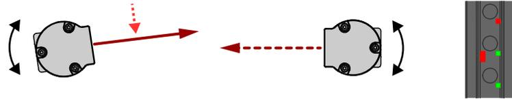
3. Optimize alignment and maximize excess gain.
