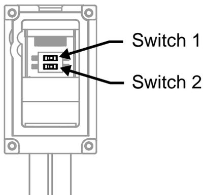
Scan Code 1: Switch 1 (top switch) in the left position
