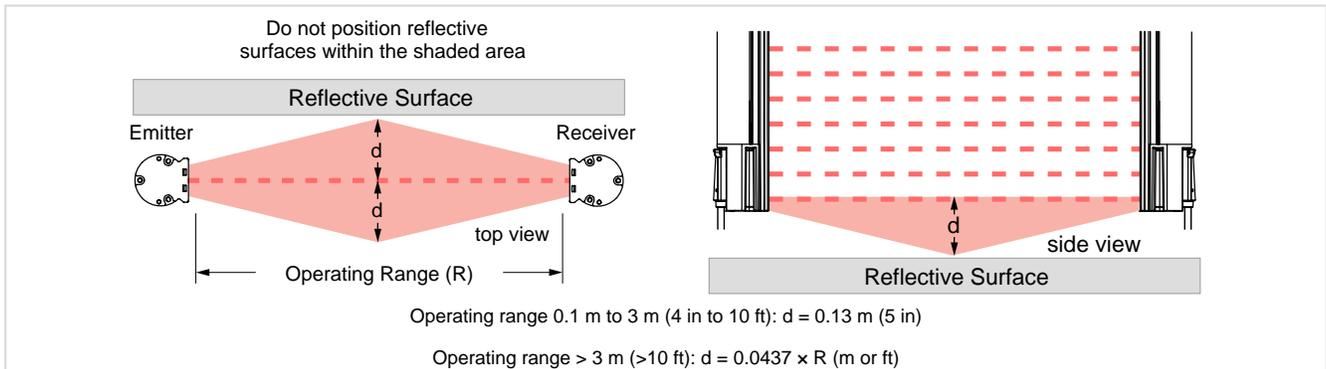
Figure 7. Determining Worst-Case Resolution With Larger Test Piece
