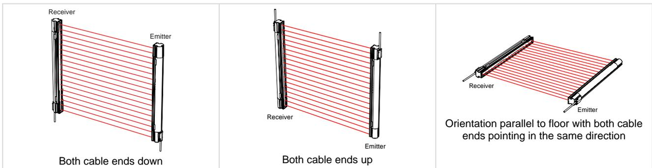
Figure 10. Examples of Incorrect Emitter/Receiver Orientation
