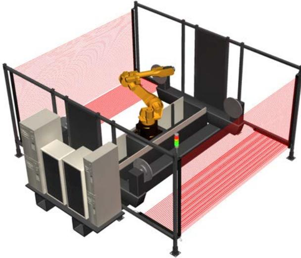
Figure 31. Cascaded light curtains guarding a u-shaped cell
