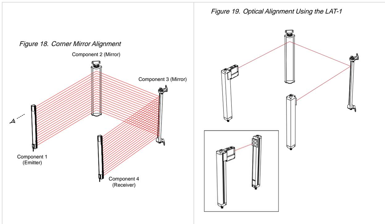
**NOTE:** An LAT-1 Laser Alignment Tool is very helpful by providing a visible red dot along the optical axis. See "[Alignment Aids](#)" on page 72 and Banner Safety Applications Note SA104 (p/n 57477) for more information.
