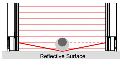
If an optical short circuit exists due to a reflective adjacent surface, a test piece (represented by the dark gray circle) with the specified system resolution will not cause a blocked condition. In this situation, during the trip test, the Zone indicators and Status indicator will be green and the OSSDs will be on.
