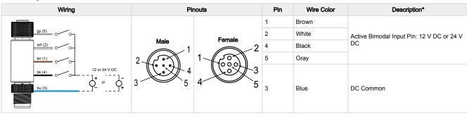
\*Continuity between male and female connection for all five wires, including IO-link communications. Each model activates from one input pin. See model table.
